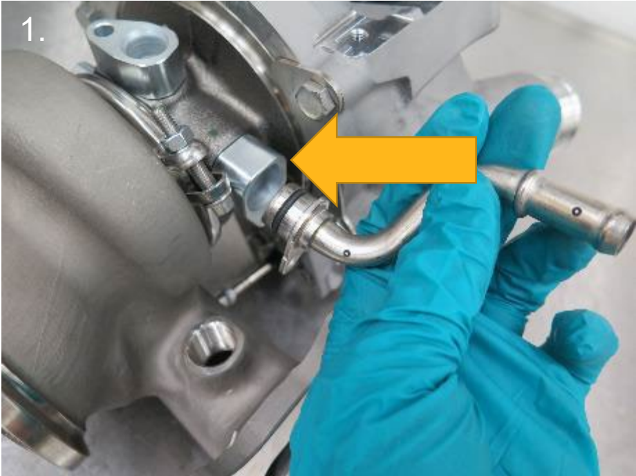
1. Lubricate water outlet pipe O-ring and press into the water outlet adapter
