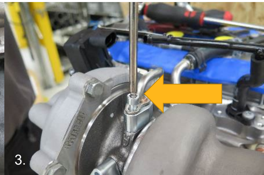
3. Tighten provided 1 M6 x 25 bolt to turbo adaptor. Torque to 7Nm / 5 ft-lb
