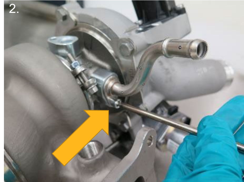
2. Attach OE water outlet pipe with provided 1 M6 x 25 bolt. Tighten to 7Nm / 5 ft-lb
