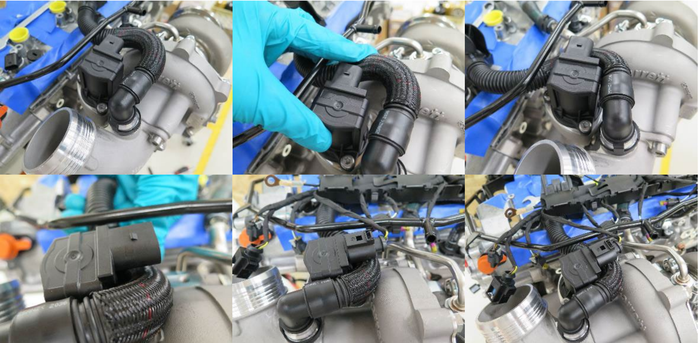
Route crankcase vent hose under electrical connector
