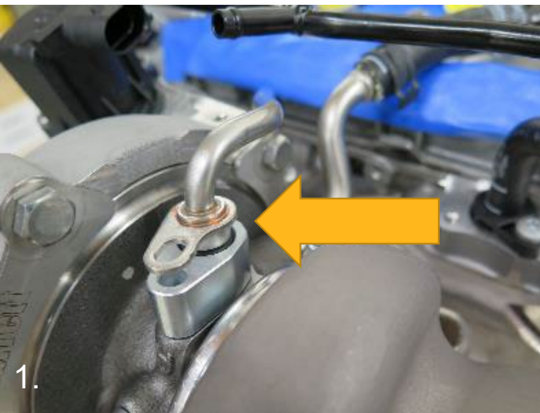
1. Attach OE oil inlet pipe to turbo adapter
