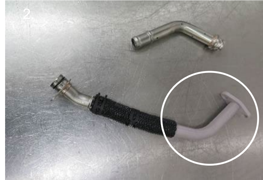
2. Replace with provided oil drain tube
