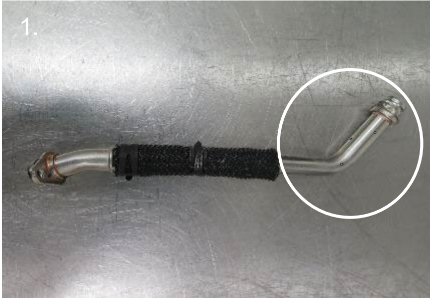
1. Remove the OEM turbo drain tube section
